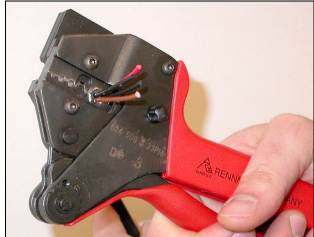
figure 45.9: Crimping the bush
